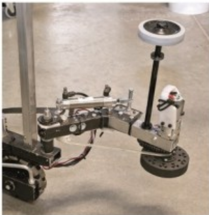
➤ A combination of sensors and mechanisms made it possible to pick up totes in any orientation.
