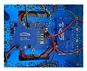
Step 27: Place the Battery in between the battery clips and connect it to the Powerpole 45 Extension Cable.
